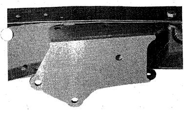
2) Enlarge rivet holes to 7/16" and drill one extra hole in the top flange of the frame to match hole in P&J mount. Bolt mount in place with grade-5 fine thread bolts & lock nuts, making sure bolts are as tight as possible! Welding mount to frame is recommended as it can move if not secure.
