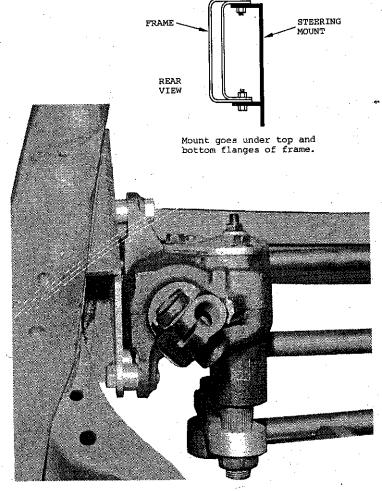
4) Bolt steering box to mount with grade-5 coarse thread bolts. Tube spacers go between mount and steering box.
