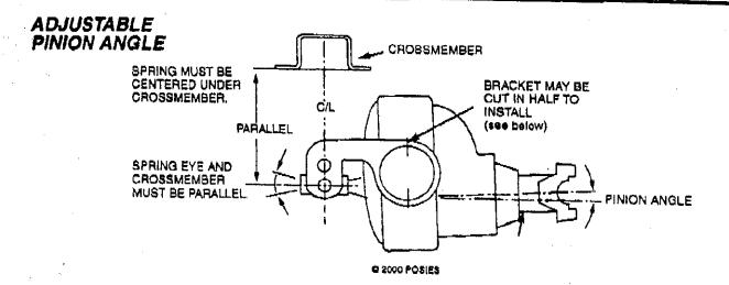
With a standard one piece spring perch, the pinion angle must be set before the perch is welded on the rear end housing. If the pinion angle must be adjusted after welding, the perch eye rotates with the axle housing, binding the spring and ruining the ride.
